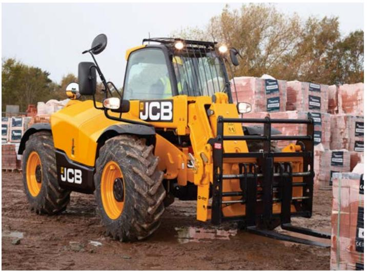
A low boom profile and pivot point, plus side and rear-view mirrors provide all-round visibility.
