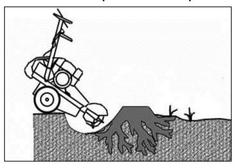
Make sure the throttle is set to "MAX". The cutter wheel is thus accelerated to cutting speed.
